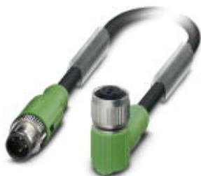
Sensor/actuator cable, 3-position, Variable cable type, shielded, Plug straight M12 SPEEDCON, A-coded, on Socket angled M12 SPEEDCON, A-coded, cable length: Free input (0.2 ... 40.0 m)
