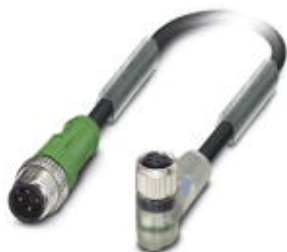
Sensor/actuator cable, 4-position, Variable cable type, Plug straight M12, A-coded, on Socket angled M8, with 2 LEDs, cable length: Free input (0.2 ... 40.0 m)
