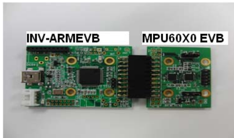
Figure 4. MPU-60X0 EVB connected to ARM Board
