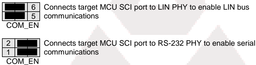
Figure 6: COM_EN Option Header
