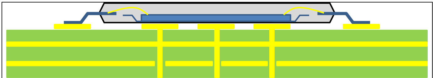
Figure 8-1: Example Thermal Via Holes on PCB.
