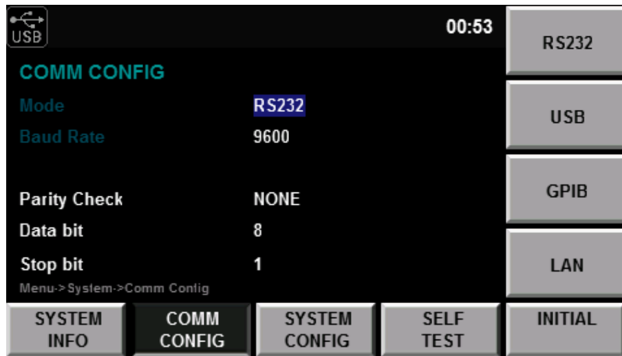
Figure 2.3: COMM Configuration - RS-232
