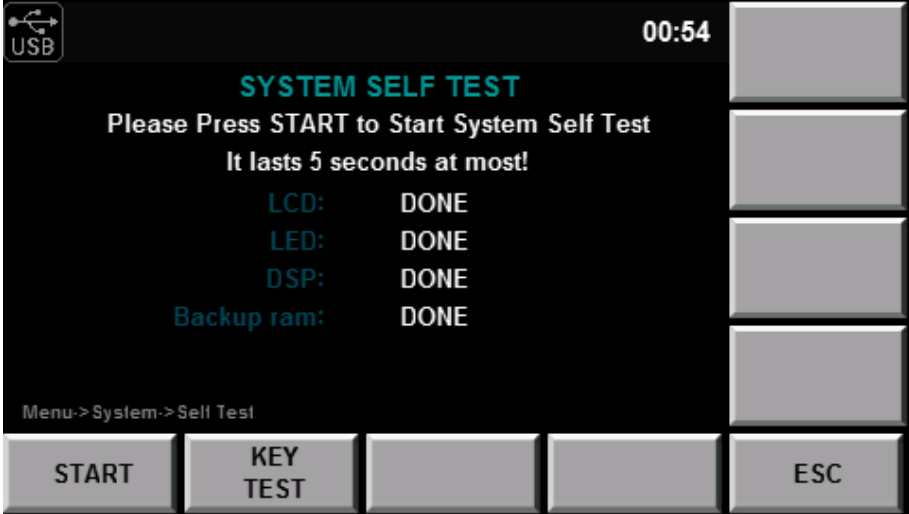
Figure 2.9: System Self Test
