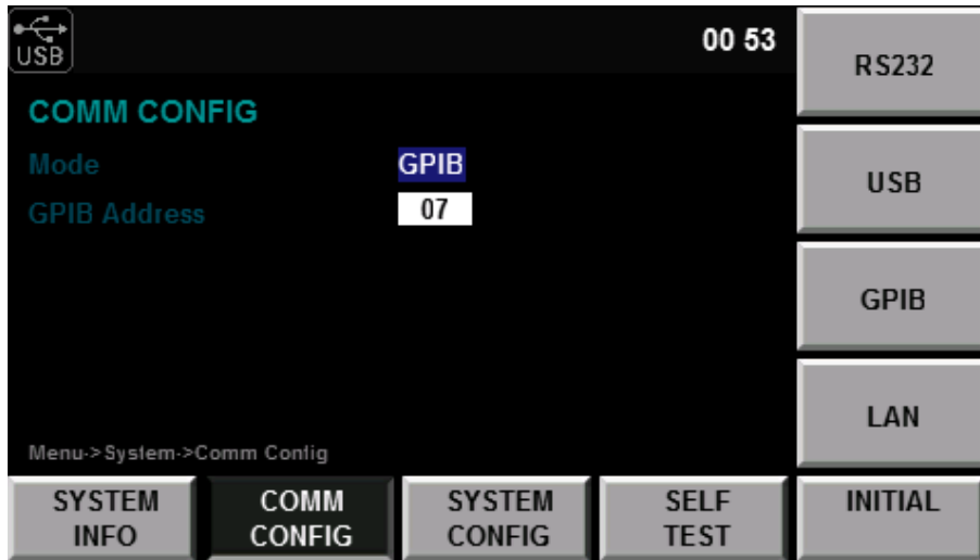
Figure 2.5: COMM Configuration - GPIB
