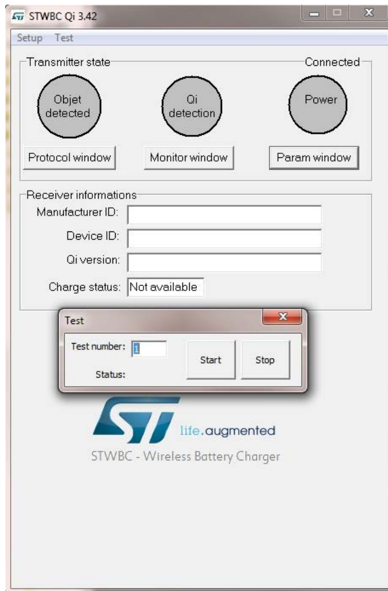
Figure 48. STSW-STWBCGUI presence detection test
