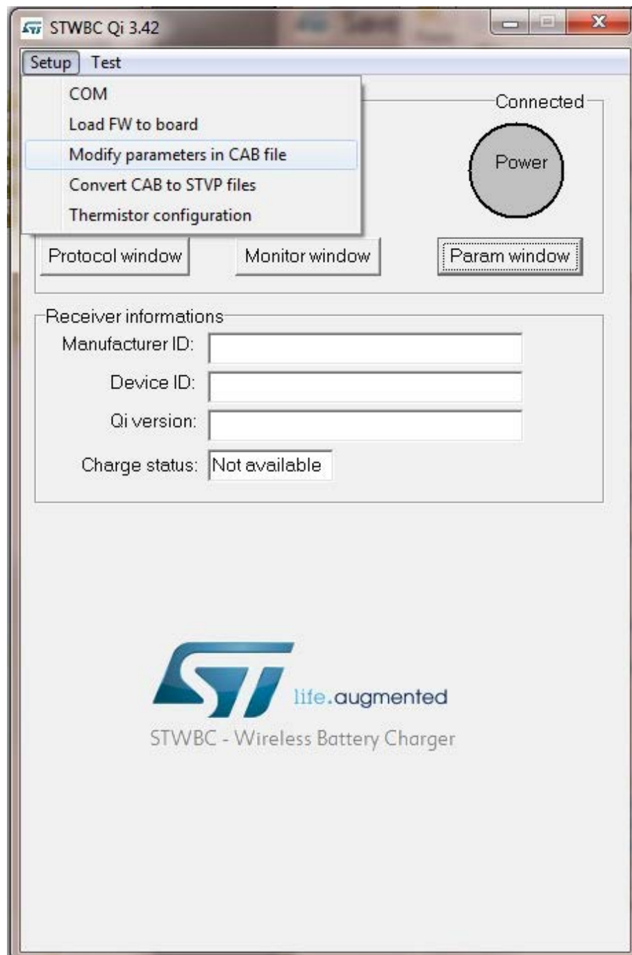
Figure 46. STSW-STWBCGUI: CAB file patch button
