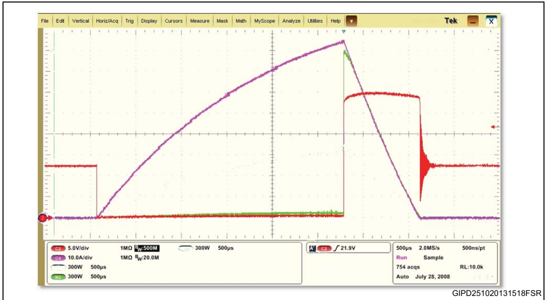
Figure 26. Unclamped inductive switching - experimental waveforms
