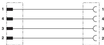
Contact assignment of M8 plugs / M12 sockets
