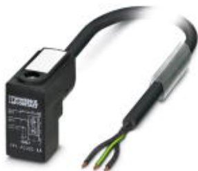
Sensor/actuator cable, 3-position, PVC, black RAL 9005, free cable end, on Valve connector CI (9.4 mm), with 1 LED, connected with Z diode, cable length: 3 m
