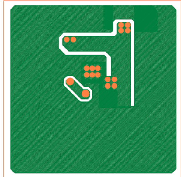
Back Side: GND Side (double sided board)
