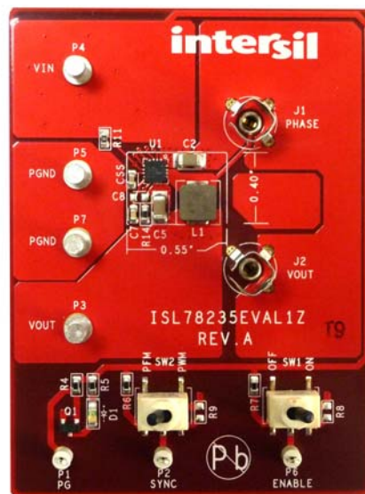
FIGURE 1. ISL78235EVAL1Z EVALUATION BOARD PHOTO
