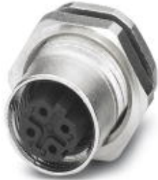
Bus system flush-type socket, ETHERNET, 4-pos., M12 SPEEDCON, D-coded, rear/screw mounting with PG9 thread, with straight solder connection
