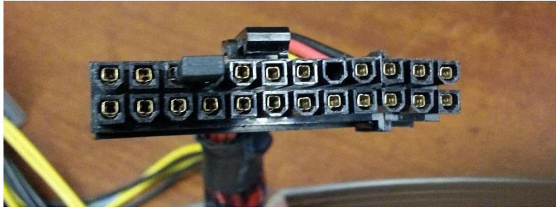
Figure 3. Pin 15 and 16 of Standard ATX power supply shorted together.
