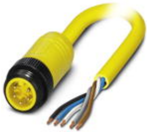
Power cable, 5-position, PVC, yellow, Plug straight 7/8"-16UNF, on free cable end, cable length: 5 m
