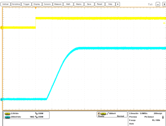
On/Off Enable Delay (Vin=5.0V, Vout=1.0V, Iout=6A, Cload=400uF) Trace1=Enable, Trace2=Vout, 2 ms/div
