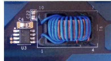
FIGURE 9. PULSE TRANSFORMER AND DRIVER
