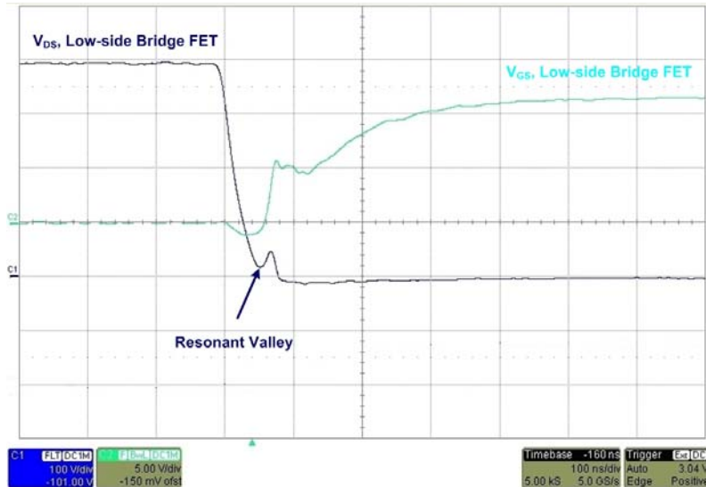
FIGURE 21. RESONANT SWITCHING WITH 100% (50A) LOAD
