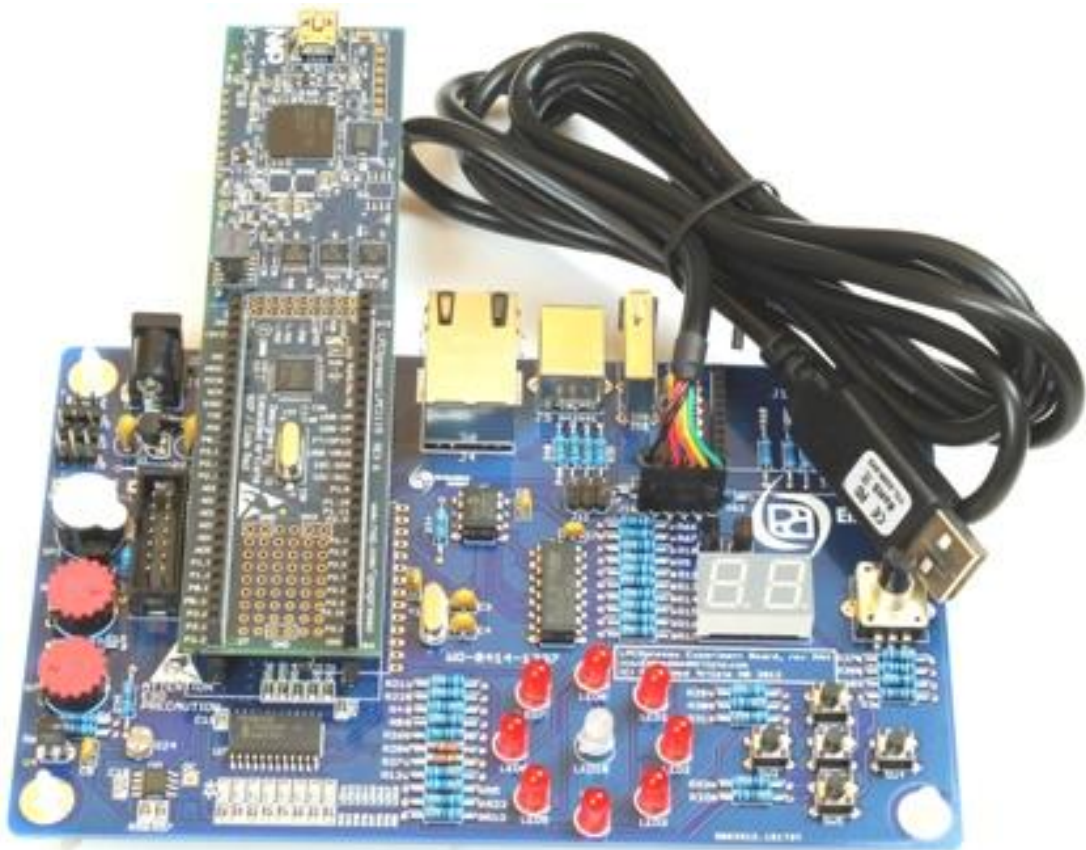
Figure 59 – LPCXpresso Experiment Kit PCB with UART-to-USB Cable
