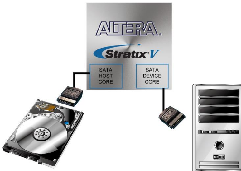
Figure 2-18 Connection between the SATA and Stratix V GX FPGA
