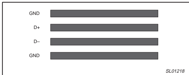
Figure 14. PCB layout for D+ and D-
