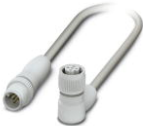
Sensor/Actuator cable, 5-position, PP-EPDM halogen-free, Gray RAL 7035, Plug straight M12, A-coded, on Socket angled M12, A-coded, Cable length: 1.5 m, Hygienic design, with plastic knurl
