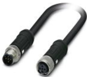
Sensor/Actuator cable, 5-position, PE-X halogen-free, black, shielded, Plug straight M12 SPEEDCON, A-coded, on Socket straight M12 SPEEDCON, A-coded, Cable length: 5 m, For railway applications
