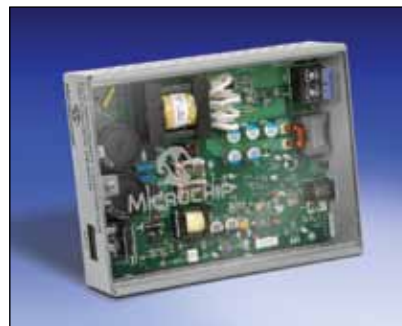
DC/DC LLC Converter Reference Design
