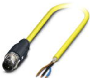
Sensor/Actuator cable, 3-position, PVC, Variable cable type, yellow, shielded, Plug straight M12 SPEEDCON, A-coded, on free cable end, Cable length: 5 m
