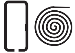
Figure 36: Loop or Trace Antenna
