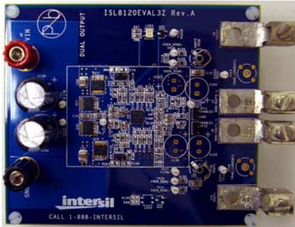
FIGURE 1. ISL8120EVAL3Z EVALUATION BOARD
