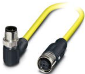
Sensor/Actuator cable, 4-position, PVC, yellow, shielded, Plug angled M12 SPEEDCON, A-coded, on Socket straight M12 SPEEDCON, A-coded, Cable length: 1.5 m
