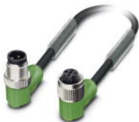
Sensor/actuator cable, 3-position, Variable cable type, Plug angled M12, A-coded, on Socket angled M12, A-coded, cable length: Free input (0.2 ... 40.0 m)
