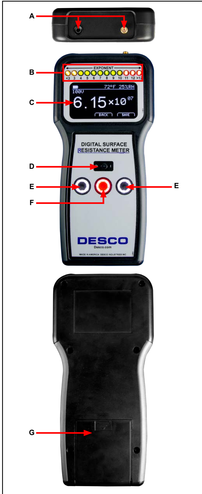
Figure 4. Digital Surface Resistance Meter features and components
